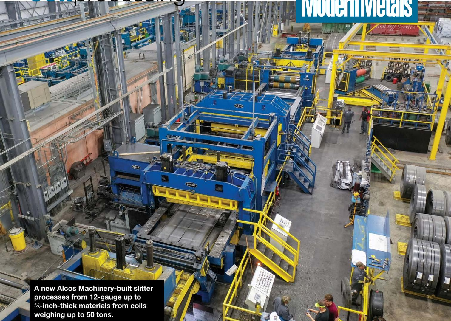
A new Alcos Machinery-built slitter processes from 12-gauge up to 5/8-inch-thick materials from coils weighing up to 50 tons.
